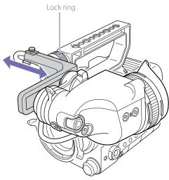
Loosen the lock ring on the camera's viewfinder shoe, and slide the unit left or right to adjust its position.
