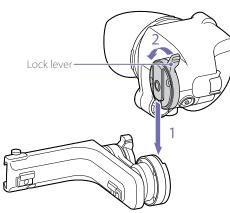
2 Connect the cable to the unit. Insert the round-type connector of the VF connection cable supplied with the CBK-55AT attachment kit (sold separately) to the VF connector of the unit.
