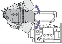
Hold the unit and adjust its angle.
