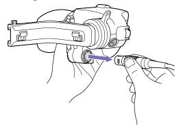
5 Turn the lock lever of the unit in the opposite direction of LOCK, and remove the unit from the CBK-55AT attachment kit (sold separately).
