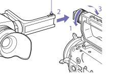
4 Connect the cable to the camera. Connect the 26-pin round type connector of the VF connection cable connected to the unit in step 2 to the camera's VF connector. Verify the orientation of the connector, and insert it until it clicks into place. Secure the cable with the clamp if necessary.
